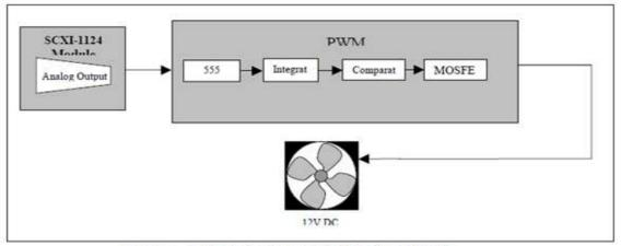
Figure 3 DC Fan Connected To Interface Circuit
