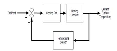
Figure 1. Feedback System Block Diagram
