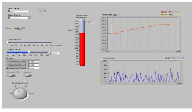
Figure 6. Autotuned PID Loop Response to Setpoint Step Change.
